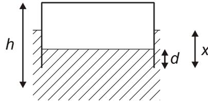
$$m_{\text{Schale}} g = \rho_{\text{Wasser}} A (x - d) g, \quad (12)$$
