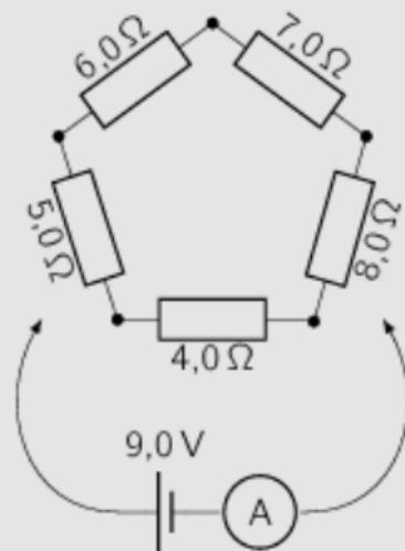
$$R = \left( \frac{1}{R_1} + \frac{1}{R_2} \right)^{-1} = \frac{R_1 R_2}{R_1 + R_2}$$
