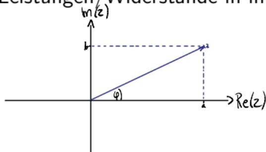
$$\begin{aligned} z &= a + ib \\ &= |z|(\cos \varphi + i \sin \varphi) \\ \Rightarrow z &= |z|e^{i\varphi} \end{aligned}$$
