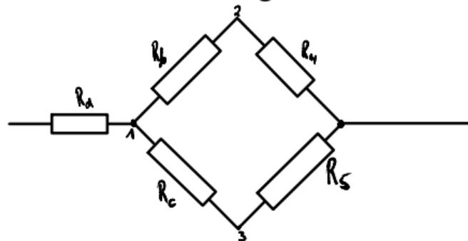
$$R_{\text{ges}} = R_a + \left( \frac{1}{R_b + R_4} + \frac{1}{R_c + R_5} \right)^{-1}$$
